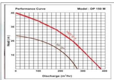
SKY 6" auto priming dewatering pump is the general purpose pump set. Designed for high volume and medium head. Excellent performance in well-point dewatering, sump pumping, transfer and treated Sewer-by- pass.
