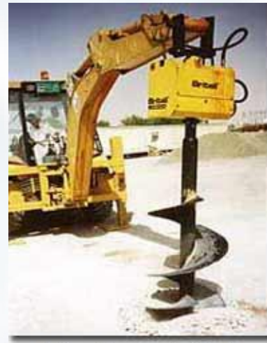
800mm Dia. x 3 metre Depth. Street-light Foundations
